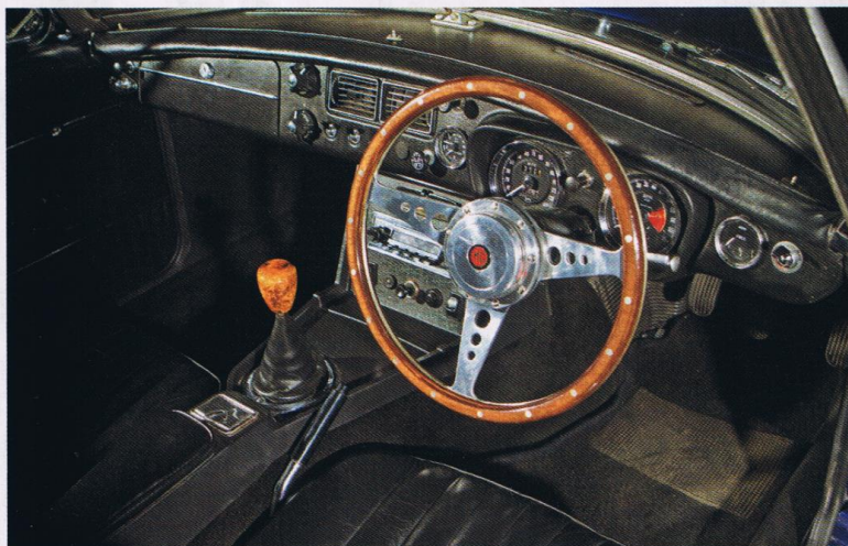
Standard dash and wood rimmed wheel, connected to a column with an extra universal joint.
